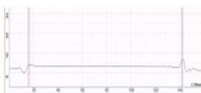
Fiber endface curvature measurement (Pre-melted before)
