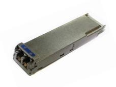
Accelink's 100Gbps QSFP28 CLR4 module is designed to meet the requirements of optical fiber interface for 2km reach over duplex SMF in data centers. It is a cost-effective, low power CWDM optical transceiver with high port densities and compact size. Each transceiver incorporates four direct modulated lasers with driver ICs, four PIN diodes with TIAs, and two Mux/De-Mux blocks in a highly integrated CWDM configuration.
