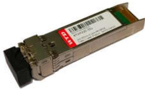
The RTX330-551 short-wavelength transceiver is designed for use in 25.78Gb/s data rate over multimode fiber. The Transceiver is compliant with SFF-8431, and the mechanical SFP+ plug is compatible with SFF-8432. Digital diagnostics functions are available via a 2-wire serial interface, as specified in SFF-8472.
