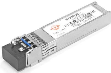
The RTX228-5XX 10Gigabit DFB laser with CWDM transceiver is designed to transmit and receive serial optical data links up from 8.5 Gb/s to 10.52 Gb/s data rate over 10km singlemode fiber. The Transceiver is compliant with SFF-8432, 10GFC, FC-PI-4, IEEE802.3ae and applicable portions of SFF-8431. Digital diagnostics functions are available via a 2-wire serial interface, as specified in SFF-8472.
